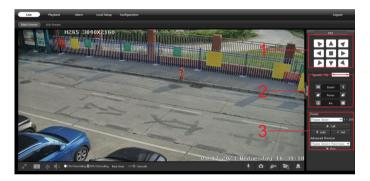
1. Rotation direction control – Left/Right horizontal rotation. Up/Down vertical rotation. Rotation speed can be adjusted.
