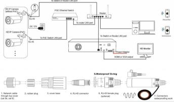
Figure 2: Working With PoE switch and NVR
