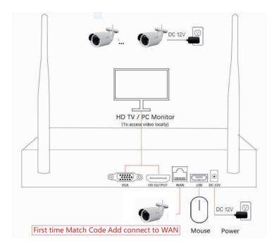
2. Click the Wifi Add button, the camera will be added to NVR automatically in 3 minutes. If nothing happen, please double-check the power and network cables connection.
