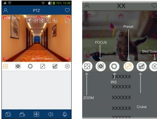
Please control the PTZ by sliding the image in direction of the arrow marked on the image. The PTZ will automatically focus on the little red circle by clicking the image. Then the 3D function can be enabled (the added device must support 3D function, or this function is ineffective).
