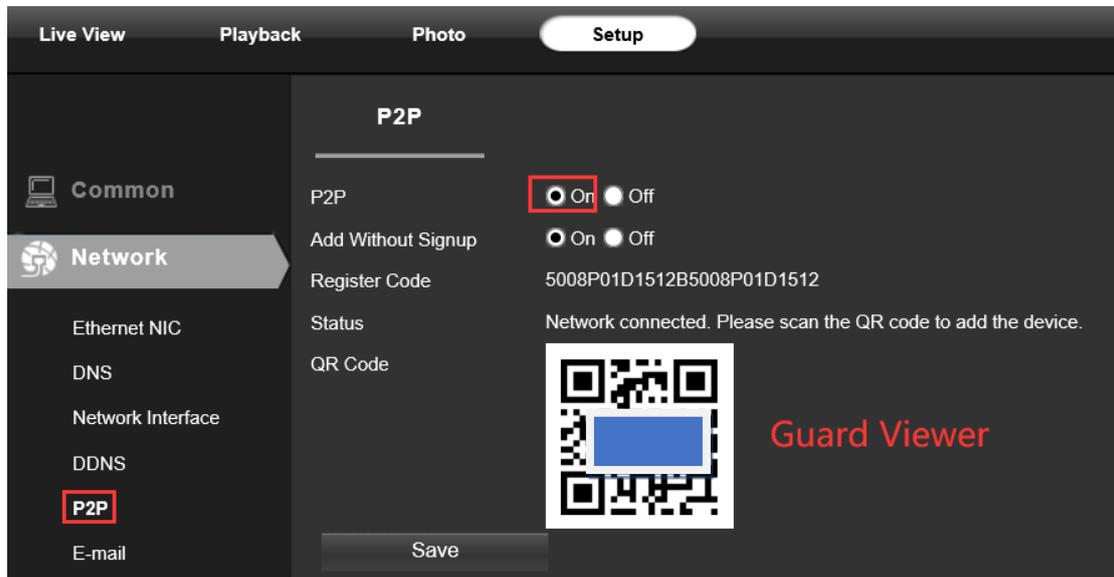
Using the P2P ID and QR code, you can access the camera remotely anywhere via smart phone with Internet access. Please register an account via mobile phone after installing the **Guard Viewer** APP from **Apple Store** or **Google Play** , then log in and add your camera to start previewing.
